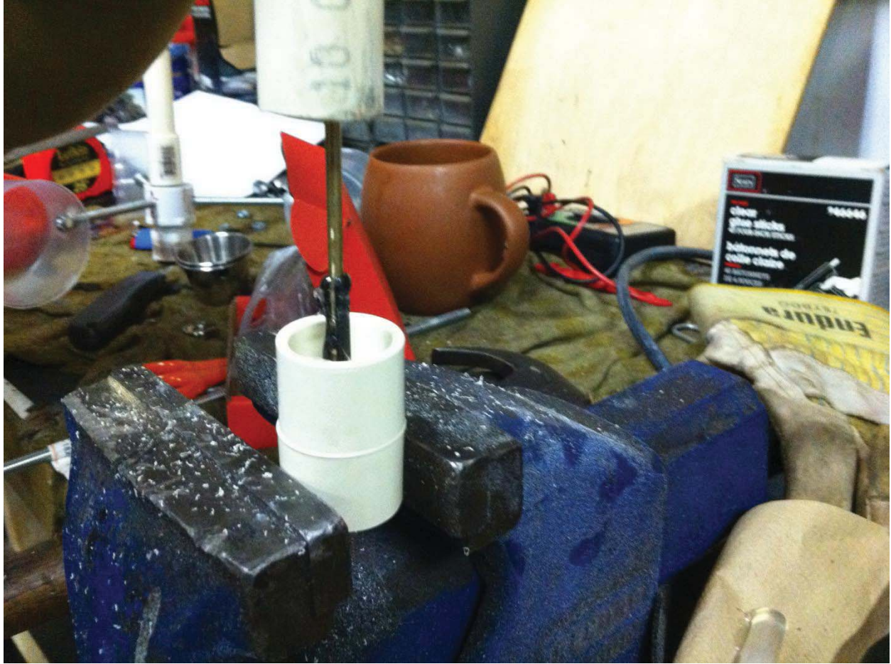
Waiting for the adhesive to set, joining the shaft of the MA3 and Wind Vane
