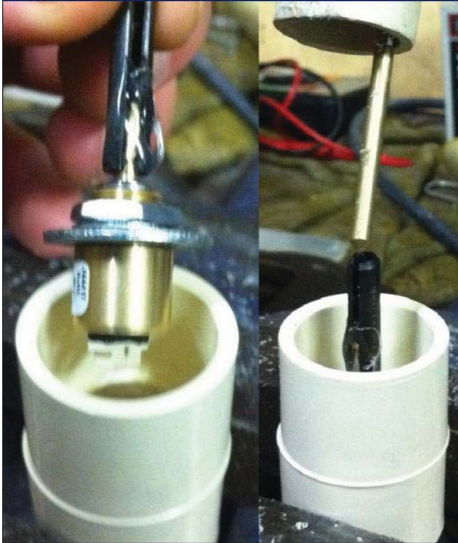
The physical construction of the wind vane
