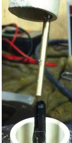
Figure 20 – Joining the MA3 shaft and Wind Vane shaft
