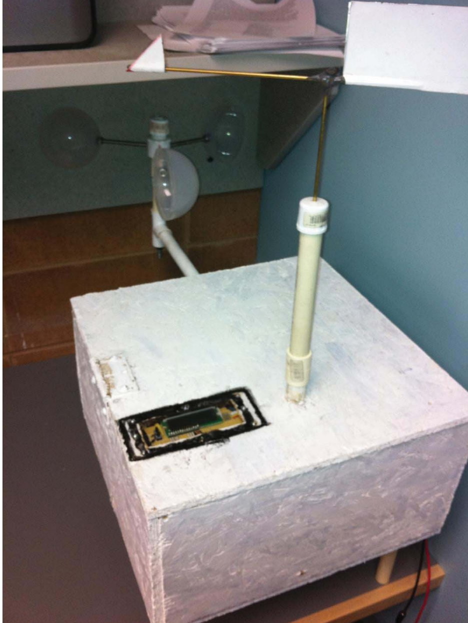
The completely assembled weather stations
