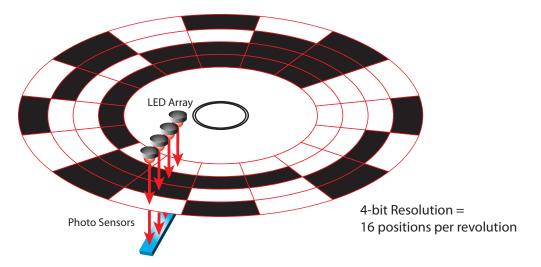
Resolution for absolute encoders is defined as the number of positions per revolution as the disk rotates through 360°. Sometimes the equivalent term codes per revolution is used.
