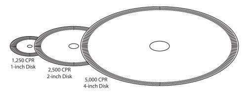
The drawing shows that, for traditional encoders, high resolution requires more lines on an encoder disk. If there's not enough space for the lines to fit, then the only solution is to make a bigger disk. To double the resolution, you have to double the disk's diameter.
