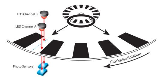
This yields a second output waveform, Channel B, shifted in phase from Channel A by 90 electrical degrees.
