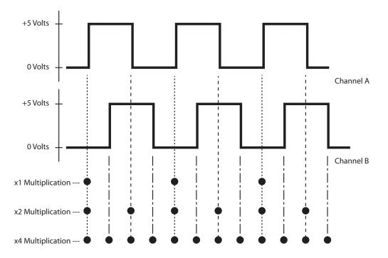
This is called *resolution multiplication*. System designers can implement it by using an encoder to counter interface chip such as an LS7183N.
