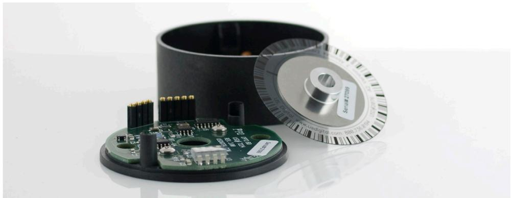
▲ *The A2K Absolute Optical Encoder can be assembled onto existing shaft and bearing assemblies. The encoder reports the shaft angle within a single 360° rotation of a shaft.*
