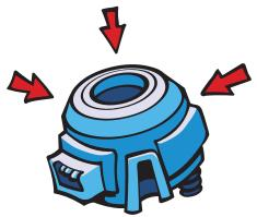
You've got a US Digital E4P kit encoder. This encoder, when mounted to the AndyMark Toughbox, is used to tell the cRio controller how fast the output shaft is turning. Knowing that info... you can effectively program the robot to move during autonomous mode!
