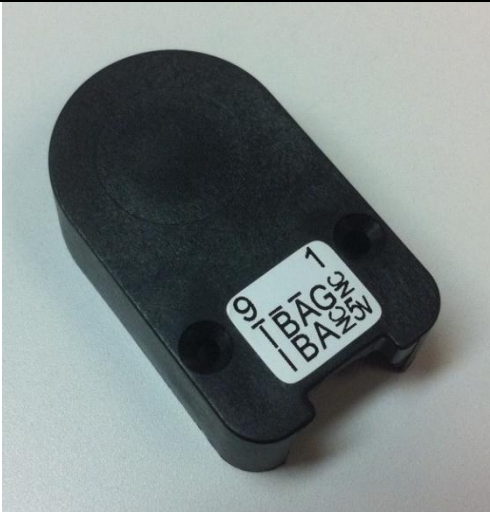
Image 3, Example of prior Avago/Agilent compatible pin-out (L) option label
